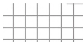
8" Quarry Tile Tile size: 195x195mm
