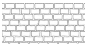
Cobble Brick Brick size: 280x140mm
